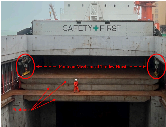
Figure 3: CH No. 2 pontoon and pontoon mechanical trolley hoist.
