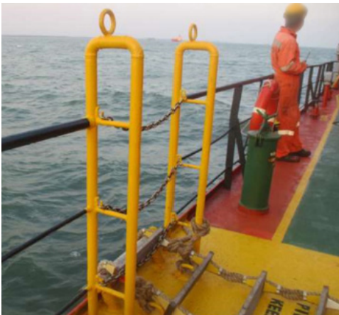
Figure 7: Starboard side pilot boarding area.
